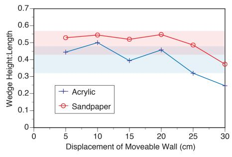
The wedge height:length seems to decrease after 20 cm of moveable wall displacement for both sandpaper and acrylic. This could mean that the end portion of our sandpaper and acrylic are more slippery than the start due to prior use.
