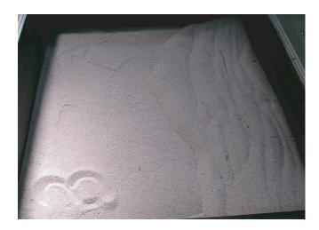
The wedge was built with 60 turns of the crank (15 cm) in compression. Wedge height is measured at the highest point -- length is measured to the toe. Note that the wedge on the 'A" acrylic side extends further into the foreland than the B side.
