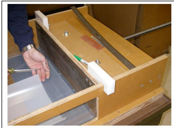
Screw mount supports: they must be glued and screwed to the lateral wall to ensure stability while cranking. 1/2" flat head screws are suitable for this:
