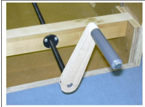
Nut for lead screw: it must be installed on one of the horizontal bars behind the moving wall. The anti-tilting bar (see apparatus design) can be added now and also glued to the moving wall. The two bars must be fastened to each other for maximum stability.
